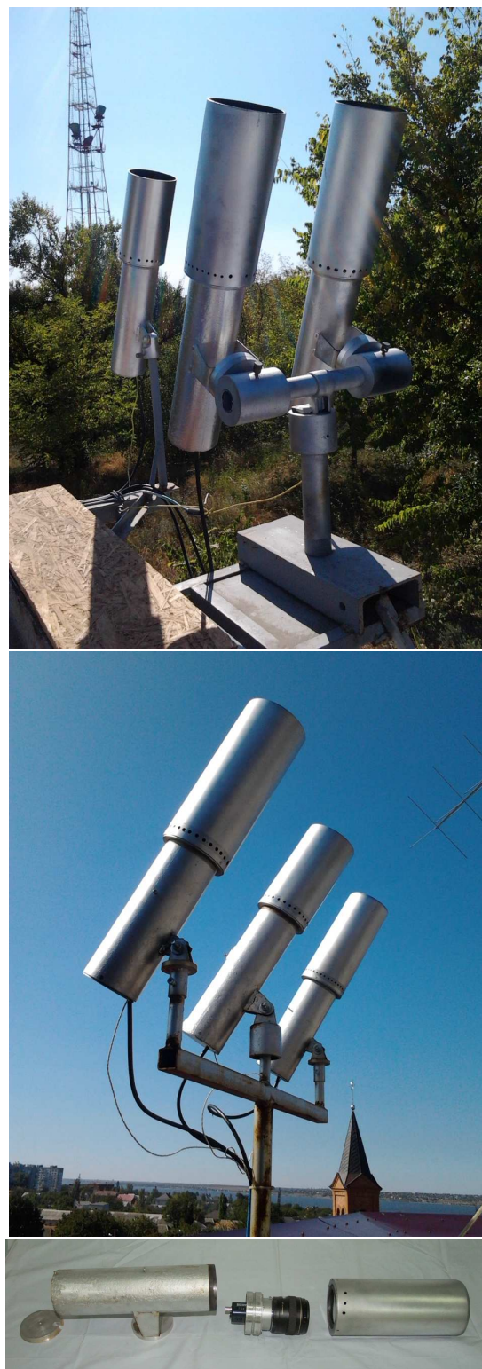
Figure 1 – Meteor patrol: a) at RI NAO; b) at station 11.8 km distant; c) meteor telescope inner housing.
